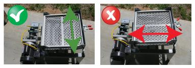
3. Place the largest screen size (Screen 1 in above table) on top of the screen already installed on the table and tighten the other clamp.
